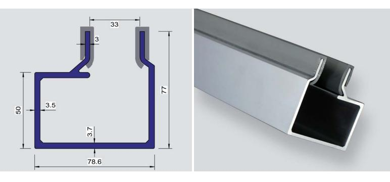
Like the prooved 1.1369 guide rail the new guide rail in extruded aluminium 1.1369 Alu can be used in combination with almost every common roller door profile. It guarantees optimal running characteristics, even for roller door shutters with storm hooks.
